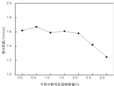
Permeability coefficients slightly decreased (0–2.0%: 1.62  $\rightarrow$  1.51 mm/s; 3.0%: 1.25 mm/s) due to pore clogging at higher dosages (Figure 4).
