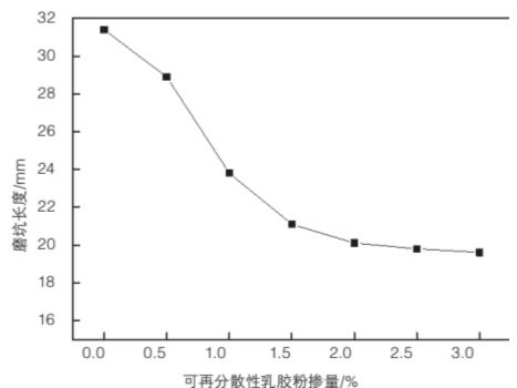
Abrasion pit length reduced with latex powder addition, plateauing beyond 2.0% (Figure 5), aligning with strength trends.
